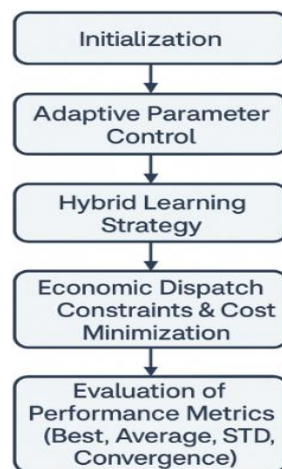
Figure 4: Process flow diagram of the modified bat algorithm for economic dispatch
